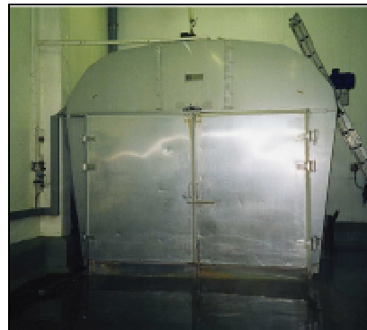
A forced air thawing unit in operation
