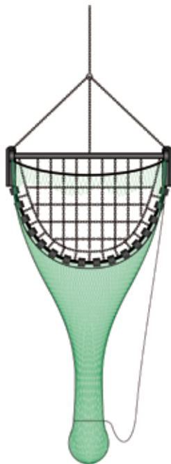
Fig 2.3 Chain mat gear
