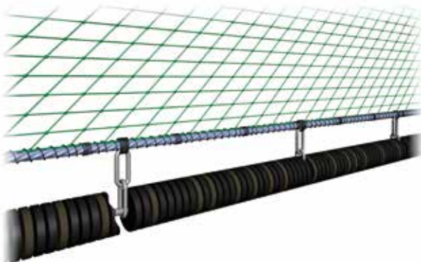
Fig 3.20 Rubber leg footrope
