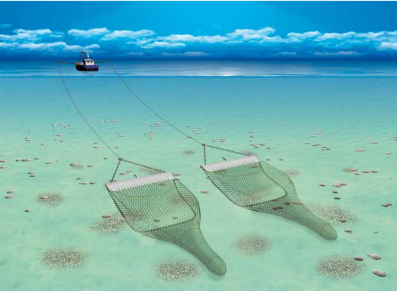
Fig 2.5 Sumwing pulse trawling
