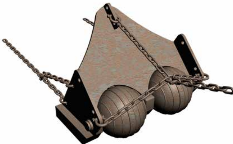
Fig 5.7 Depressor clump weight
