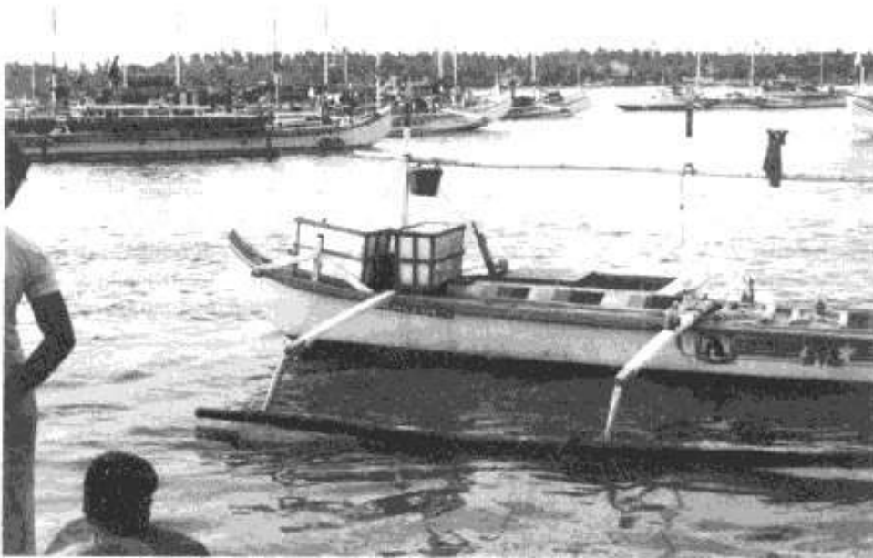
Figure 7.10 Small insulated container installed onboard an artisanal fish catamaran (The Philippines, 1982, photo H. Lupin)
