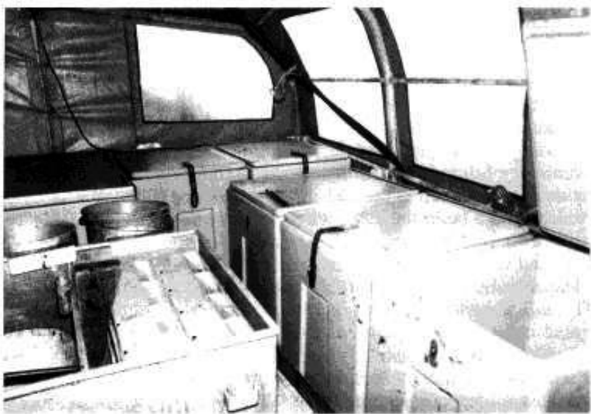
Figure 7.19 Some of the 10 pieces of 200 l CSW containers placed on deck on a 15 GRT cod gillnet wooden boat
