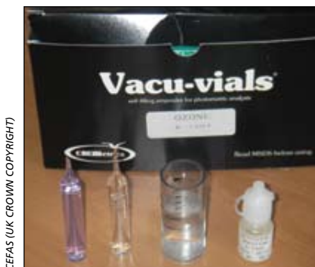
Figure 8.2: Example of a kit for the measurement of ozone
