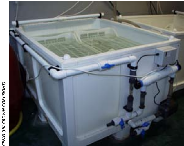
Figure 5.4: The standard design small-scale shallow tank system
